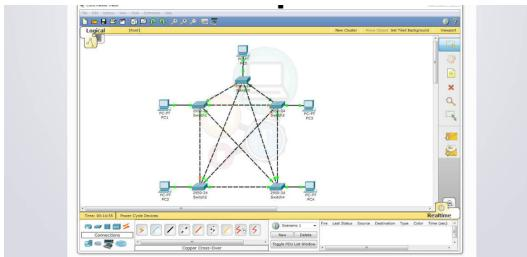
Now, each switch has a dedicated connection to every other one so you don't need to make any further connections. All the devices are connected and you can see the **mesh network structure** clearly.
